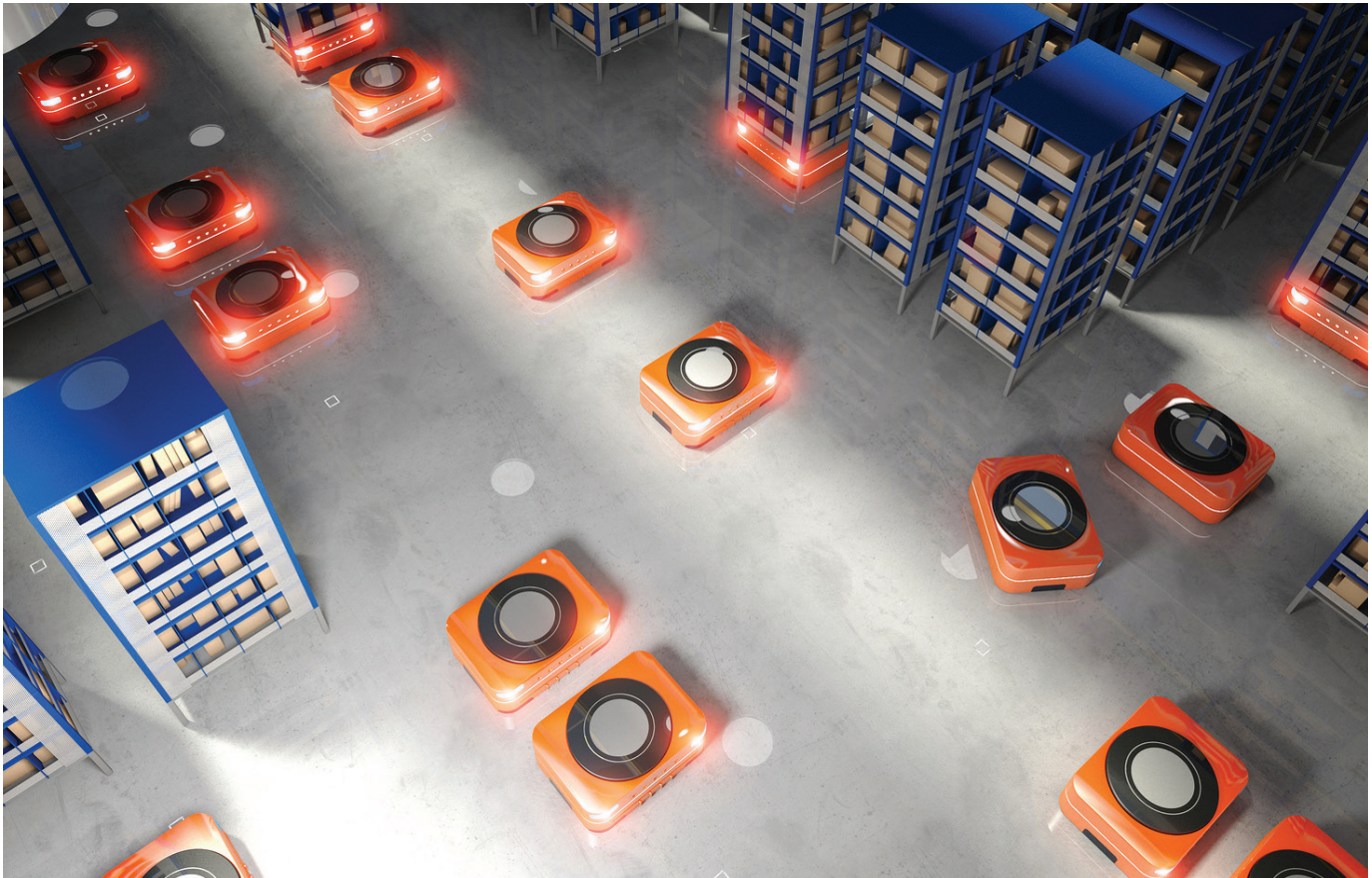
In 2012, Amazon bought Kiva Systems (now Amazon Robotics), which designed these robots specifically for warehouses
